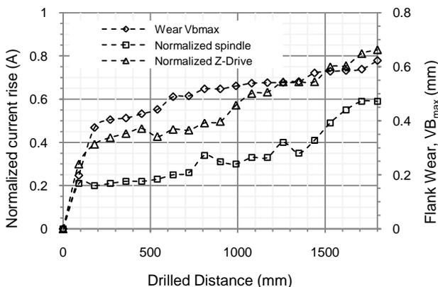
**FIGURE 3: Normalized spindle current (RMS) and Z-drive current vs. drilled distance for a TERA drill (test case C2). Progressive flank-wear,  $VB_{max}$ , values are also plotted on the secondary axis.**
