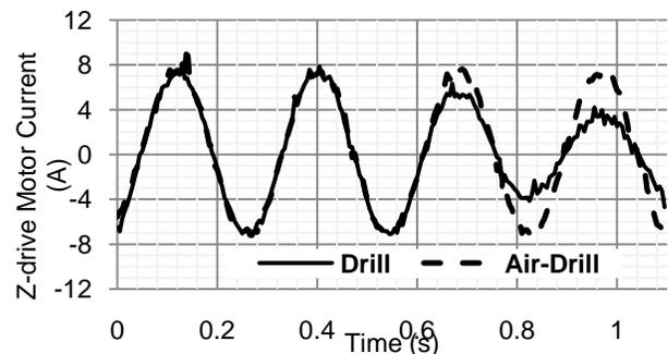
**FIGURE 1: Z-drive motor’s true current for a typical signal (one full motor cycle = 0.28 second) generated from an actual drilling test superimposed on another corresponding to an air-drilling test (both for the same parameters: test case B3, drilled distance 7.524 m).**
