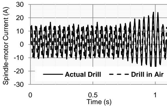
**FIGURE 2: Spindle-motor true current for a typical signal (one full motor cycle = 0.28 second) generated from an actual drilling test superimposed on another corresponding to an air-drilling test (both for the same parameters: test case B3, drilled distance 7.524 m).**
